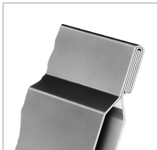
Fig. C5: Double fold connections give the exchanger package several-fold material thickness for the leading and trailing edges
