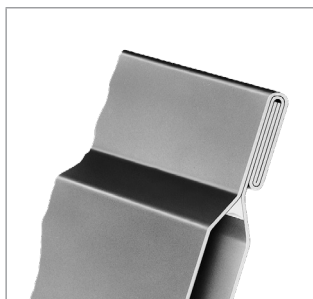
Fig. D3: Double fold connections give the exchanger package several-fold material thickness for the leading and trailing edges
