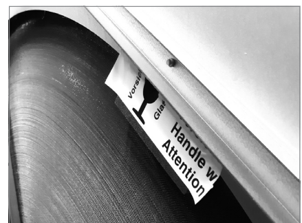
Fig. 52: Removing transport protections
