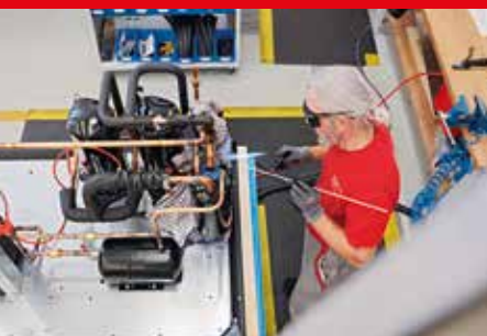
Installation of the refrigeration circuit
